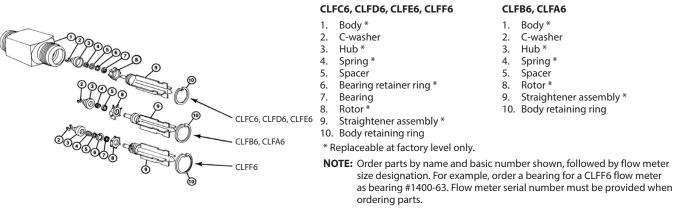
Figure 1: Cox Precision LoFlo turbine flow meter
