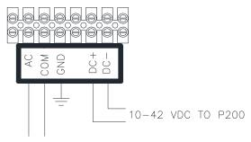
120 VAC FOR: L100A/L100AR (TIMER & SOLENOID VALVES) L22 OPTION (DIGITAL READOUT)
