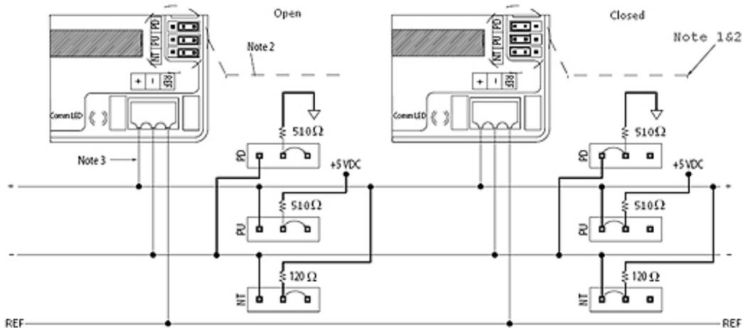
Figure 13: Sample wiring diagram to modbus network
