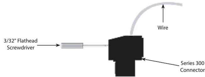
Figure 7: Side View - Typical series 300 removable connector wiring
