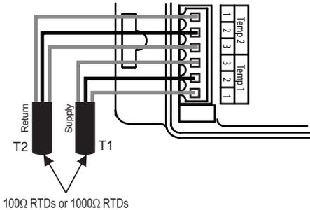
Figure 11: RTD wiring diagram
