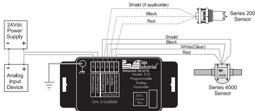
Figure 5: Typical wiring example
