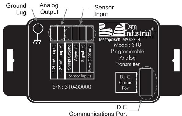
Figure 4: Terminal connections
