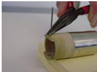
4. Flip the sensor over so that it is resting on the flat section of the electronics assembly, and the tip remains supported. This will provide a stable working platform for Step #5.
