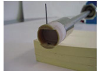
6. Carefully position a new impeller so that the stub end of the new shaft is starting to enter the bearing. Continue to drive the shaft through the first bearing and then carefully guide it into and then through the second. Once through the bearing carefully guide the shaft through the hole in the other side of the impeller cavity.
