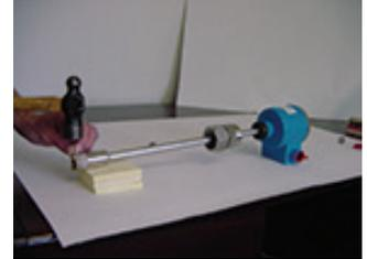
5. Use small hammer and one of the new shafts to drive the remaining shaft end into the center of the impeller cavity. Drive the new shaft all the way through the cavity wall until the old shaft fragment drops out and about 1/32" of the new shaft is exposed in the cavity. In this picture the old shaft fragment is shown resting on the lower impeller cavity wall.
