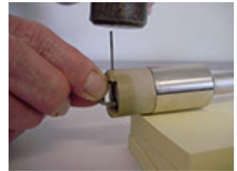
7. Continue to drive the shaft until it is flush with the plastic housing.
