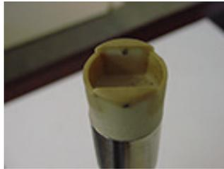
2. Lay the sensor on a flat surface with the flat portion of the electronics housing facing up, and the metal part of the sensor tip supported high enough that the tip lays horizontal. This will make it easier to drive the remaining shaft ends out of the tip.
