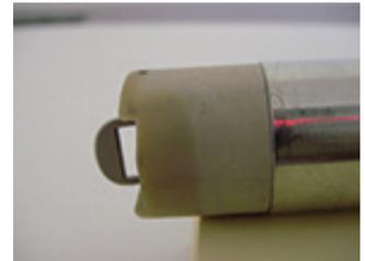
Installation is now complete. If done properly, when spun by hand, the impeller will spin freely on the shaft, and glide smoothly to a stop.
