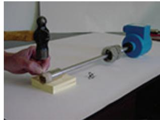
3. Using a small hammer and one of the new shafts, carefully drive the first remaining shaft end into the center of the impeller cavity. Drive the new shaft in only as far as necessary to be able to grab the old shaft with a pair of needle nose pliers. Carefully work the shaft end out with the pliers. Again using the pliers, work the new shaft back out.
