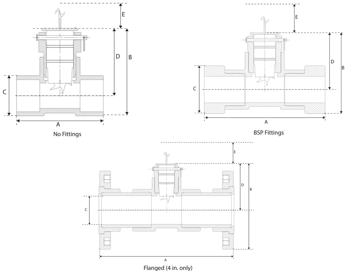
Figure 1: A = Overall Length; B = Overall Height; C = Diameter; D = Center of Tube to Top Height; E = Minimum Clearance for Sensor Removal
