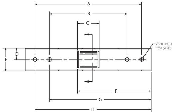
Figure 5: RCTN pipe bracket dimensions
