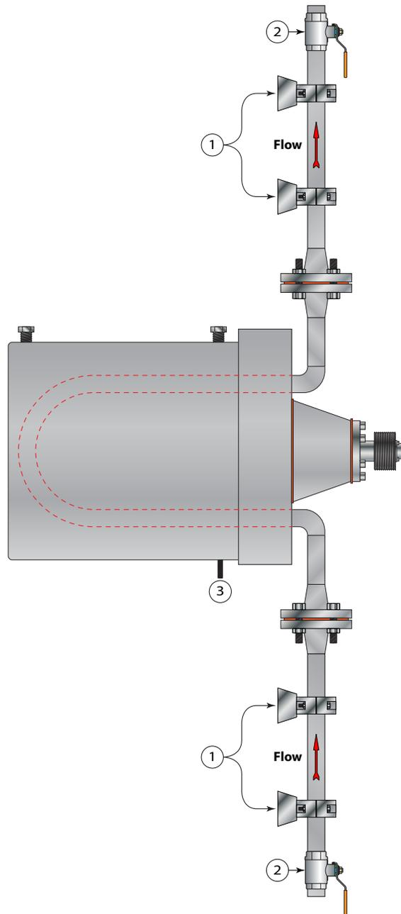
Figure 9: Tubes to the side with flow going up (self-draining)
