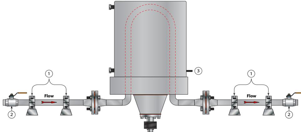
Figure 10: Tubes up (slurries)
