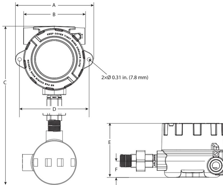
Figure 2: RCTX remote mount dimensions
