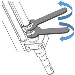
Figure 6: Removing the hex nut
