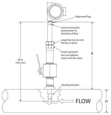
Figure 3: Calculate insertion depth
