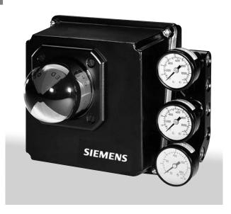
A spool valve is used to load the actuator for positioning in response to an input signal. A characterized cam provides mechanical feedback. There are linear, equal percentage and quick opening operation cam profiles, and a blank profile cam is available for custom applications. Rectilinear action length can range from 1/2" to 6".
