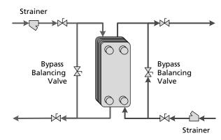
Typical Piping Arrangement Involving a Cooling Tower
