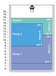
The pump alternation feature of the Vantage 2200 is utilized when the treatment facility has more than two pumps that are to be actuated based upon level set points.
